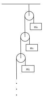
An infinite series of pulleys and masses is arranged as shown, with  $m_0 = 1/(1-t)$ , and  $m_i = t^{(i-1)}$  for i > 0, with 0 < t < 1. At the moment the pulleys are released from rest, what is the acceleration of mass  $m_0$ ?
