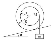
A bobbin of M = 3 kg consists of a central cylinder of radius r = 5 cm and two end plates of radius R = 6 cm. It is placed on a slotted incline on which it will roll but not slip, and a mass m = 4.5 kg is suspended from a cord wound around the bobbin. It is observed that the system is in static equilibrium. What is the angle of tilt  $\theta$  of the incline?
